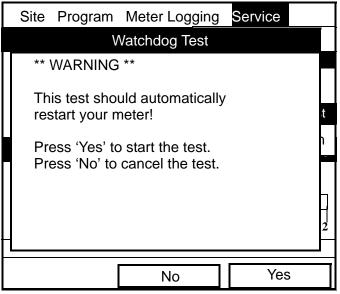
Figure 126: Watchdog Test Screen
